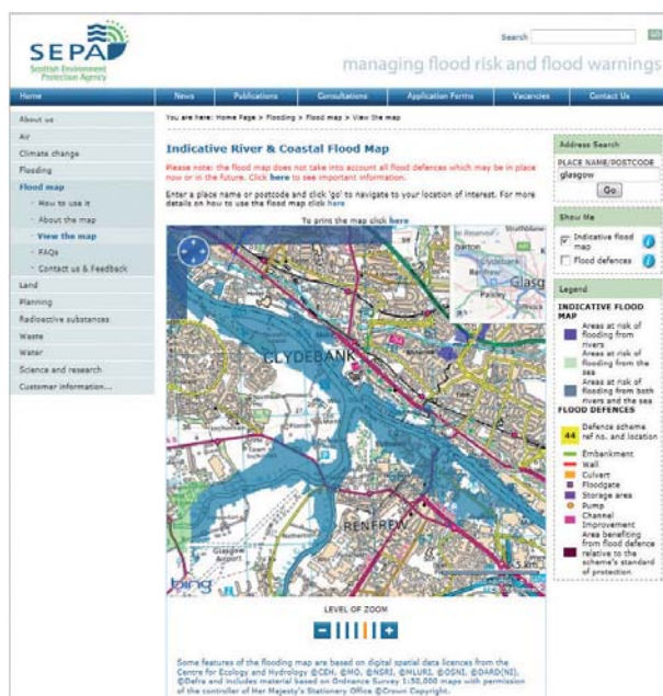
Figure 82: Example of an undefended flood hazard map for the 1:100 year fluvial flow event as publicly disseminated through a web service in Scotland
