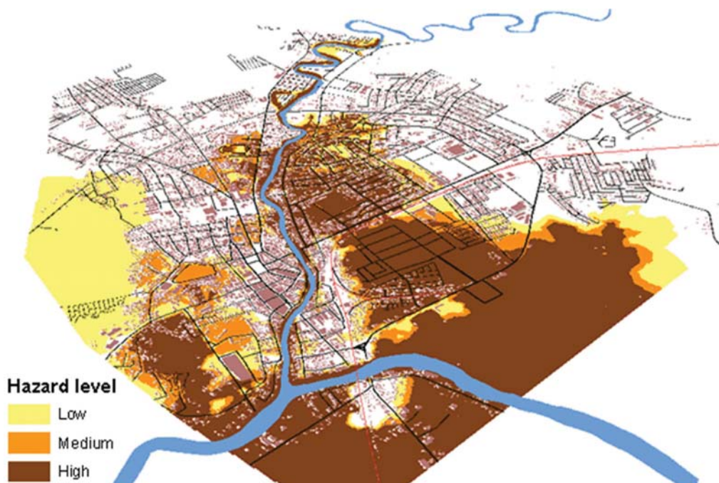
Figure 75: Naga, Philippines: spatial variation in flood depth is used to zone development in the floodplain
